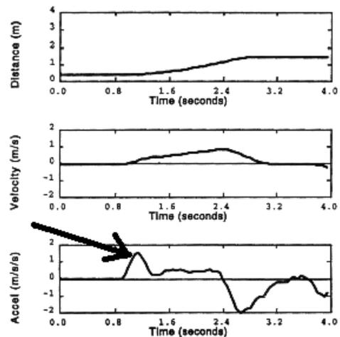
At the start of the first lesson following the interview Martin approached the teacher and suggested a second possibility, that the trolley's back wheel had been 'choked' with a piece of wood. When pulled over the chock, the trolley had a larger initial acceleration, which would explain the bump. Martin's explanation reflected considerable insight into the meaning of the graph, and a singular cognitive engagement with the earlier MBL activities.
